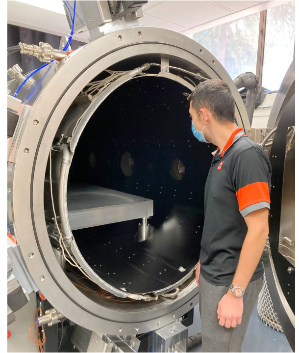
Student Kian Milani inspecting the vacuum space simulation chamber in the basement of Steward Observatory. Photo credit: Lori Harrison
